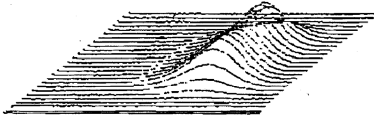
Figure 3. Eddy Current Scans of 12.54-mm Crack in Specimen J71
