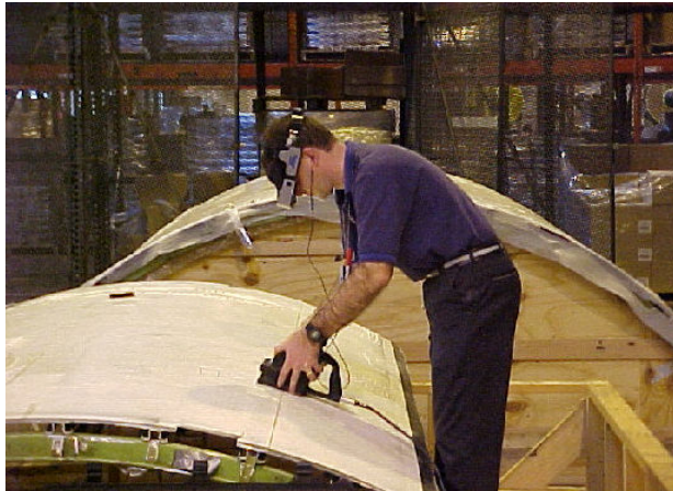
External MOI NDT under controlled conditions after panel removal.
