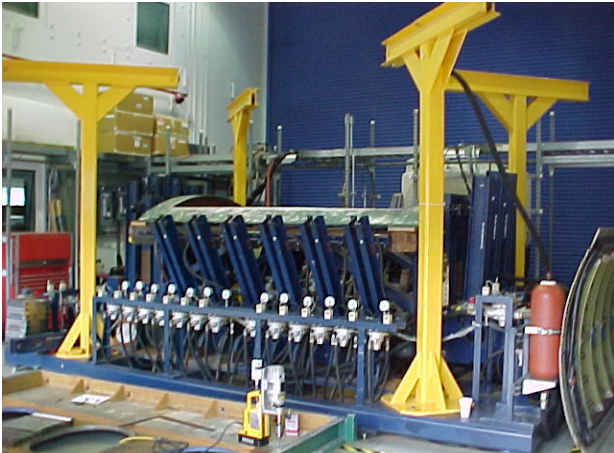
FASTER fixture prior to panel installation. Shows top of pressure box, hoop loader, and shear fixture counterweight frames
