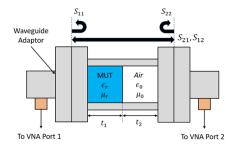
• The material properties are obtained from measured S-Parameters using a model of the filled waveguide and an optimization algorithm.
