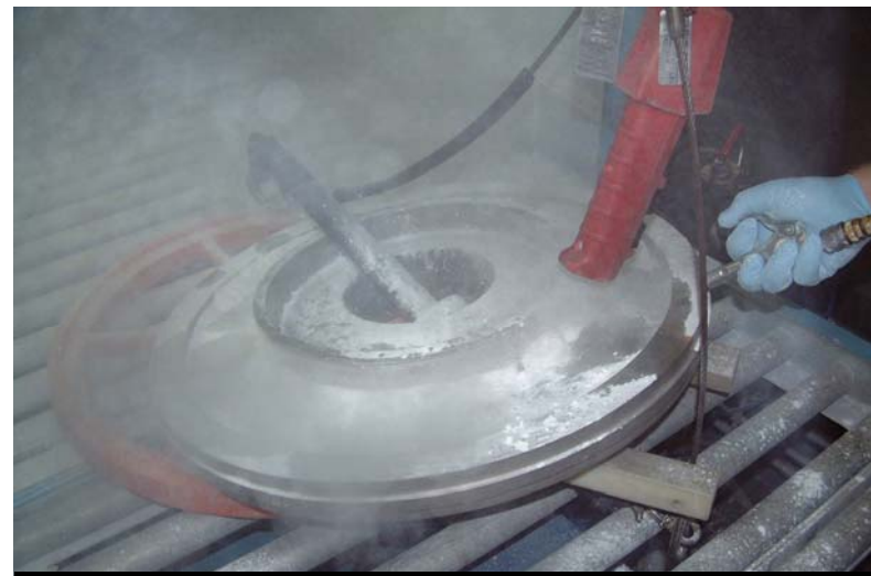
Removal of excess developer powder
