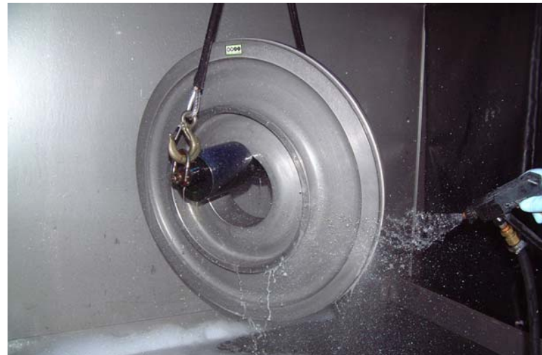
Final spray rinse, 60 sec
