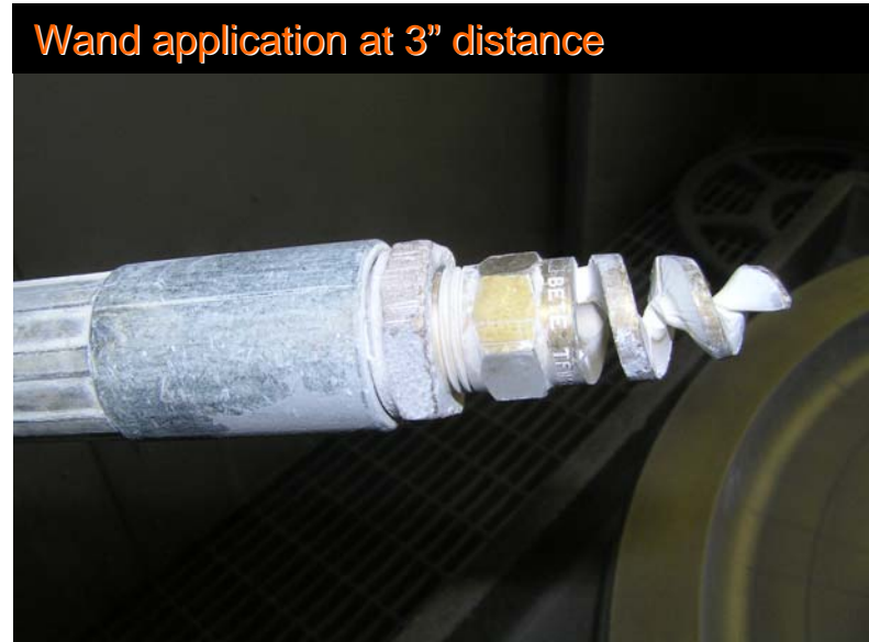
Dry developer applied with force
