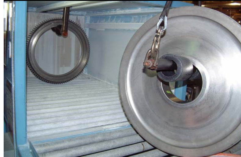
Developer application in dust chamber
