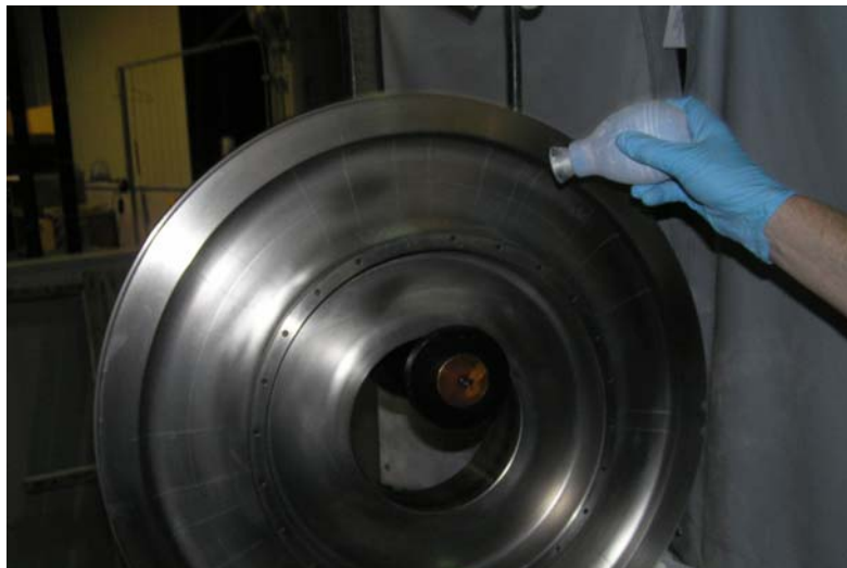
Bulb application of dry powder developer
