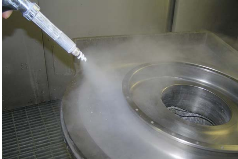
Wand application at 3" distance
