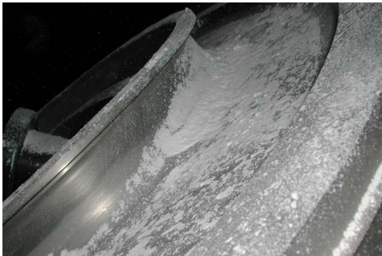
Hand application by tossing of dry powder
