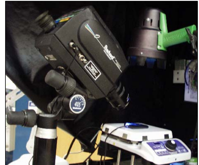
Photometer, UVA source, and digital hotplate used for some runs
