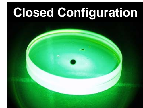
Two-disc penetrant sandwich effectively removing air interaction
