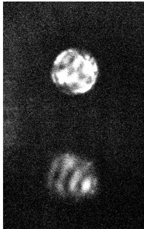
Figure 3. A thermosonic image of a 12-ply glass-fiber skin over a Nomex core. The two simulated defects are believed to be a pillow insert (top) and a region of potted core (bottom).
