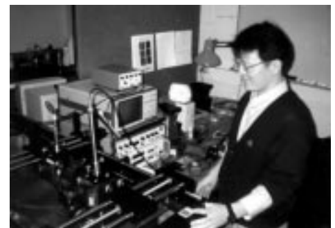
Yohan Rew of Samsung Heavy Industries conducting ultrasonic measurements in the composite nondestructive evaluation laboratory at CNDE. ■
