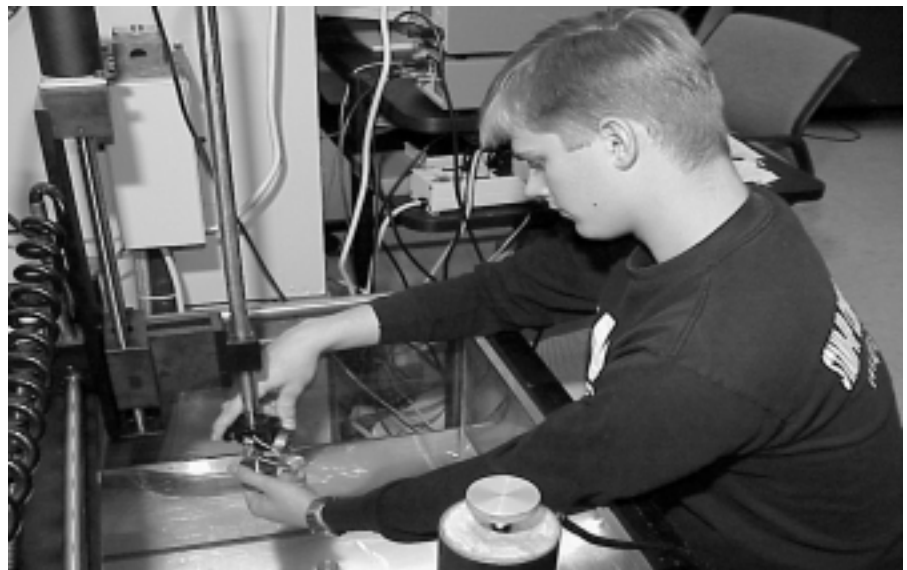
Engineering student Zach Nielsen examines corrosion on an airplane wing in an ultrasonic immersion tank at the Center for Nondestructive Evaluation. Materials science and engineering students will engage in similar advanced computer and life-cycle testing projects through the new Combined Research and Curriculum Development Program.
